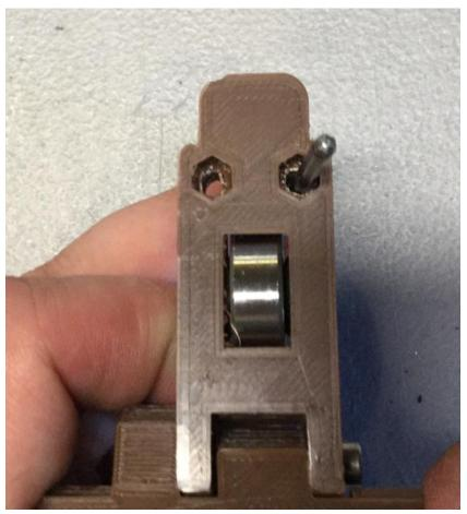
Install two M4 nuts in the nut traps shown by the Red Arrows
