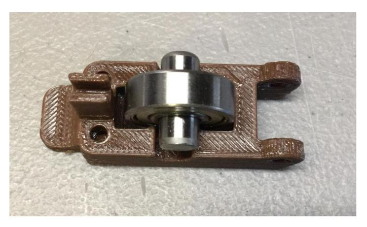
Install the dowel rod into the 608 bearing align them onto the Guidler then push the dowel rod in place as shown below.
