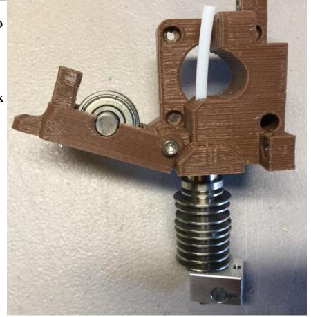
Next we will cut the PTFE Tube so its goes just past the extruder block, make sure you push the hot end as far into the extruder block as possible before cutting the ptfe tube.
