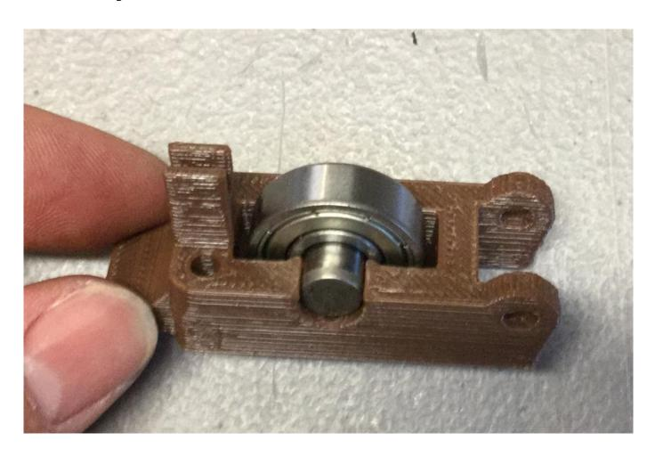
Install the Guidler onto the extruder block and secure using the M3x30mm bolt and regular M3 nut as shown below.
