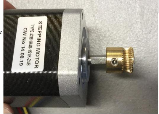
Install the Nema 17 motor using the 4 M3x10mm long bolts.
