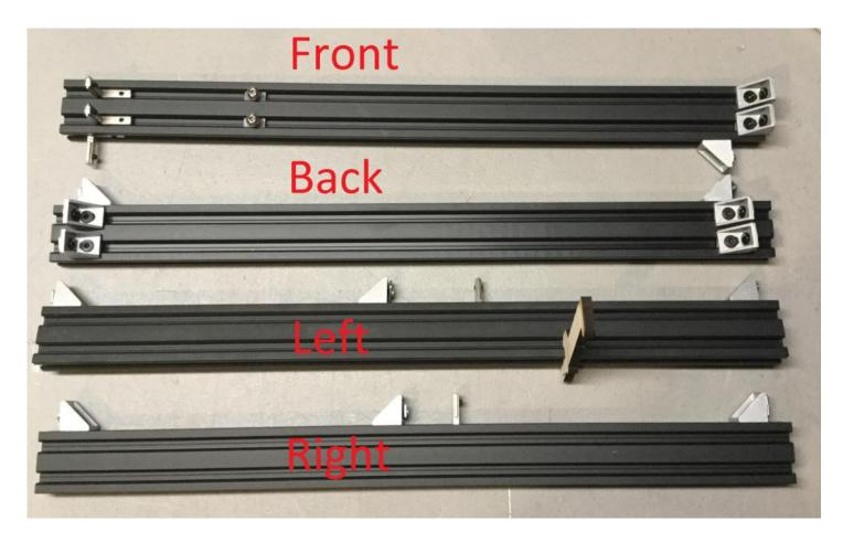
For this section you are assembling the top part of the frame upside down so it will lay flat during assembly.
