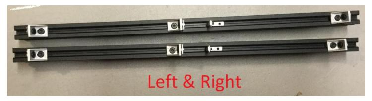
2. Next get 2 more extrusions, Install an M5x8mm Bolt and T-Slot Nut in the 6 locations shown with green arrows. Get 2 Cast Corner Brackets, 2 M5x8mm Bolts and 2 T-Slot Nuts and install them in the center of the Front Extrusion as shown by the Red Arrows. Get 12 Cast Corner Brackets, 24 M5x8mm Bolts and 24 T-Slot Nuts, Install them on the ends of the two extrusions so your Front and Back Extrusions match the picture below.
