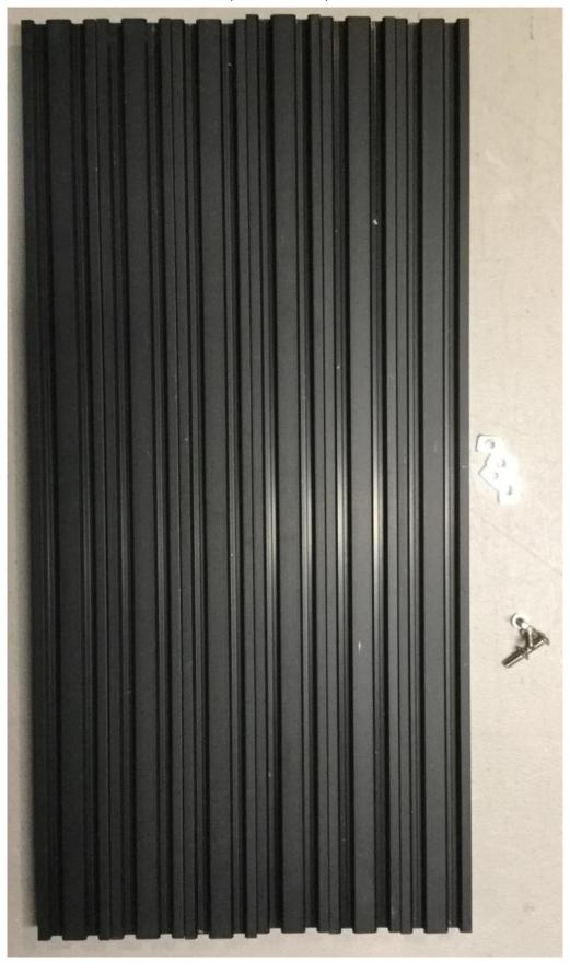
Install an M5x12mm bolt and T-Slot Nut on 3 of the Extrusions as shown below.
