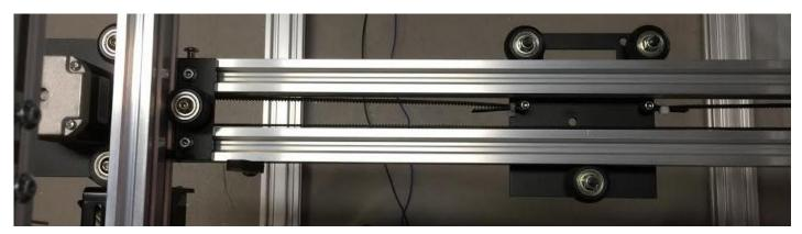
At this time you can also adjust the Eccentric Spacer on the X carriage so all 3 wheels contact the Aluminum Extrusion.
