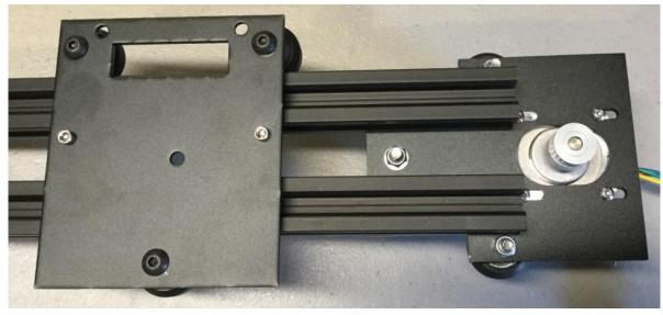
Install a M5x12mm bolt with a T-Slot nut into the top extrusion as shown by the Red Arrow, then Install one M5x12mm bolt and T-Slot nut into the two Z Nut traps and install them as shown by the Blue Arrows, Last slide the X Idler Bracket onto the back of the Extrusion as shown by the Green Arrow. (Leave the X idler loose)
