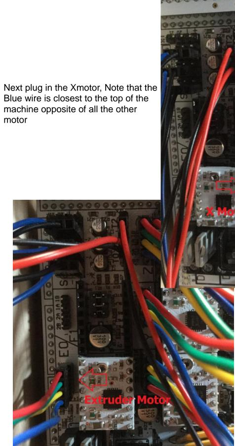
Now plug in the Extruder Motor (Single Extruder motor will plug into the E0 port, Dual Extruder Right Extruder motor will plug in to E0, Left Extruder will Plug into E1) If your heat bed has 4 wires, connect the small heat bed wires to D8 on your electronics shown by the Blue Arrow below. If your heat bed has 2 wires then follow this guide to install the heat bed relay: <u>Heat Bed Relay Guide</u>
