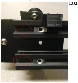
Install the Belt Idler onto the two T-Slots using two M5x12mm long bolts, The Belt Idler bolt will go into the hole in the X Idler bracket
