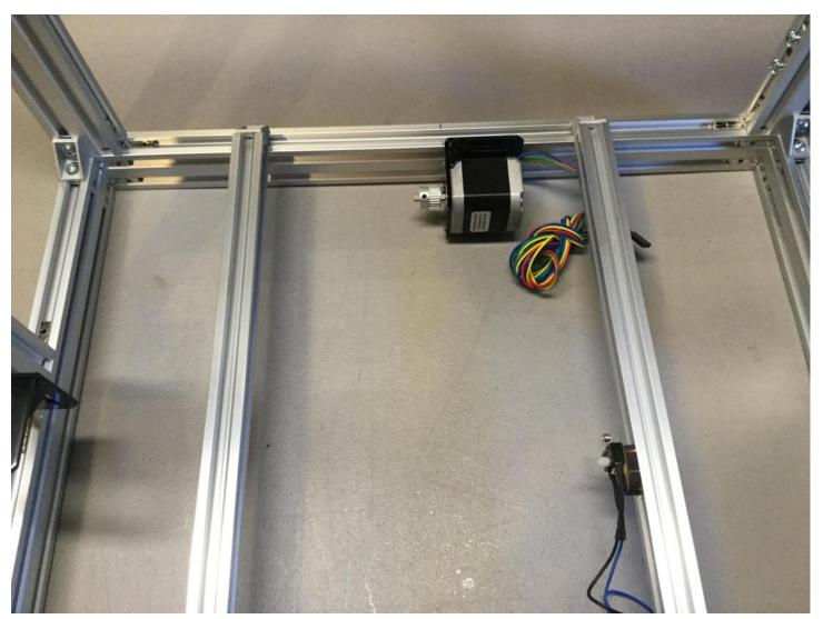
Adjust the two Z motor mounts so the surface the Z motor contacts is 55mm above the extrusion as
