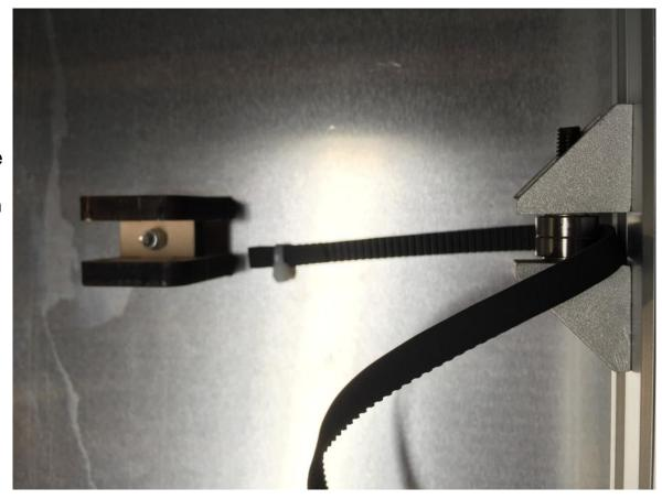
around the GT2 Gear then back to the wooden mount, Loop the other end making sure that the belt will be tight when you install it into the wooden mount, then zip tie the loop and install the loop to the wooden mount using the other M3 bolt and Nylon Lock nut.
