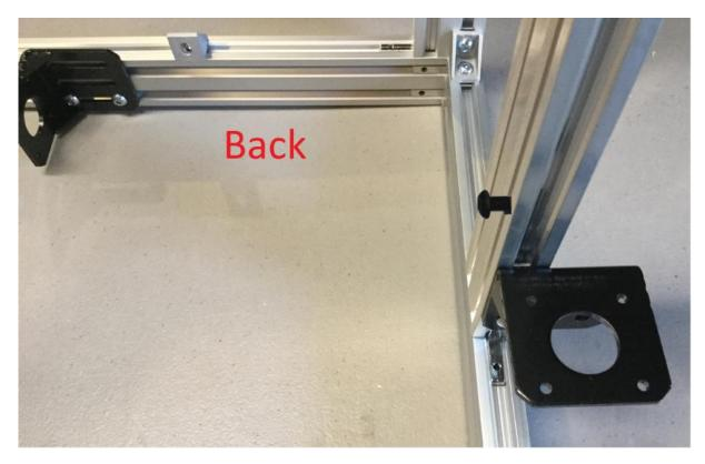
Now Install a Motor Mount of the left side of the printer, make sure you use the slot on the far left of the motor bracket.
