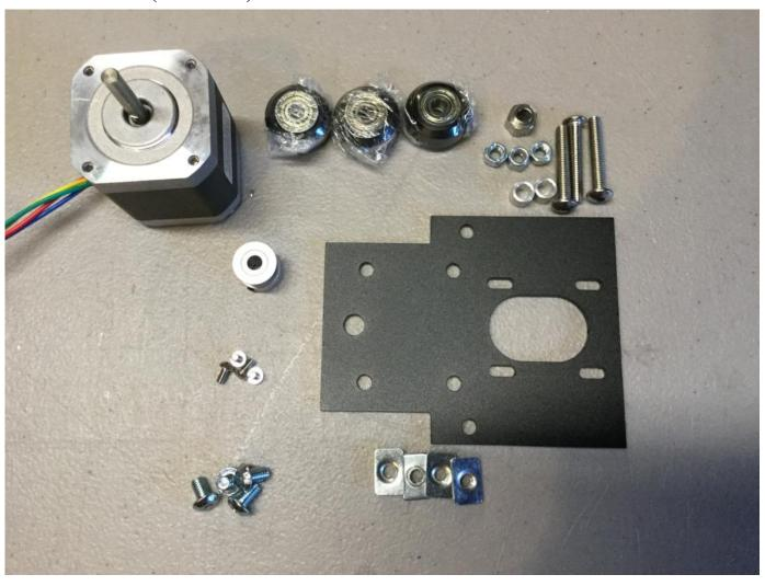
Install 4 M5x8mm bolts in to the Metal from the back then install a T-Slot Nut on each of the 4 bolts
