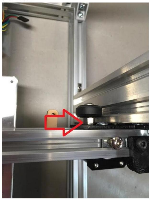
Now tighten the Eccentric spacer on the X Idler side so all 3 delrin wheels contact the extrusion, then tighten down all the bolts holding the X idler and Belt idler to the extrusion.
