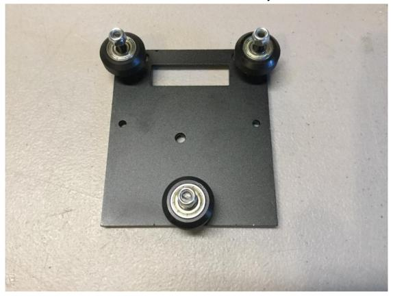
Last Install the two M3x16mm Bolts and regular M3 nuts as shown, tighten them down. Then loosly install the Nylon Lock nuts on the M3 bolts, you will remove them later to install the X Belt.
