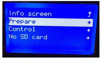
Then turn the knob until the arrow points at "Level Bed" then push the knob. The printer will home then the nozzle will move to the position shown below. Turn the knob until the nozzle just barely touches the glass then push the knob. The printer will then move to 8 other locations, turn the knob to move the nozzle up or down then when it just barely touches the glass push the knob again.
