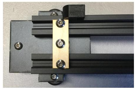
Now slide the X axis down onto the Frame as shown below. Since your X idler bolts are loose you can adjust the placement of the X idler to allow the X axis to slide onto the extrusion.
