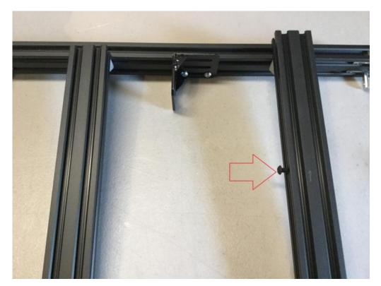
Connect the extrusion to the Cast Corner Brackets in the front of the machine also.
