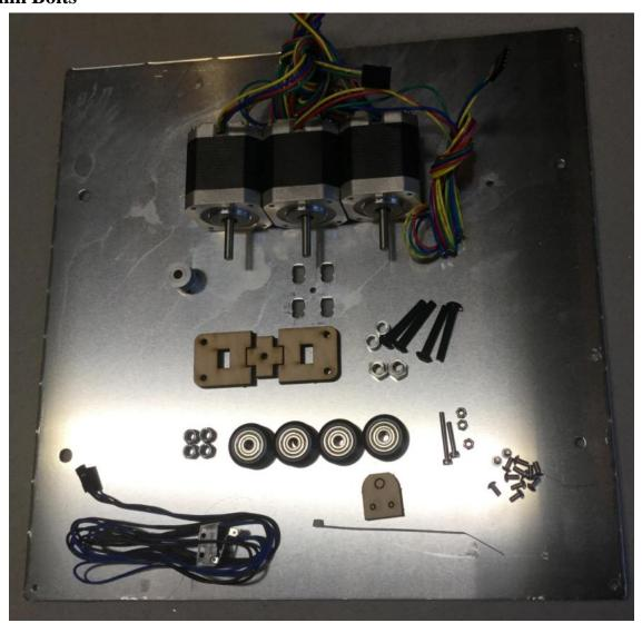
To start install a GT2 gear onto a motor as shown below, make sure to align one of the set screws with the flat spot on the Motor.
