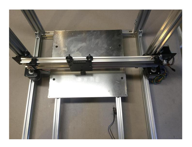
While the bolts that hold the X idler side to the extrusion are loose turn the eccentric spacer on the X motor until you can see that all 3 delrin wheels on the X motor contact the extrusion.
