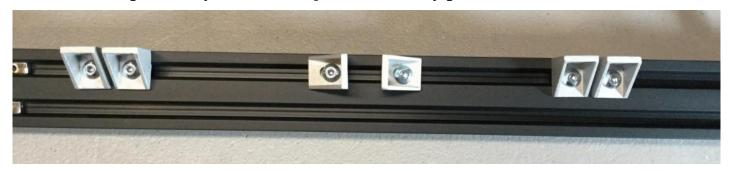
Now install 4 Cast Corner Brackets and one Motor Mount on the bottom back of the frame using the previously installed M5x8mm Bolts. You will adjust the actually placement later.
