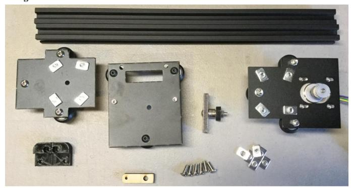
Slide the two Extrusions onto the T-Slot nuts on the X Motor Bracket, push the extrusions away from each other inbetween the two T-Slot nuts then tighten the bolts down, your Extrusions should now be parallel to each other. Slide the X Carriage onto the extrusion as shown below.
