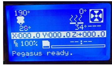
Go back to "Control", "Temperature", change the bed temp to 0 then change the hot end temperature to 190c. Now go back to the "Info Screen" and verify that the hot end temp is rising.
