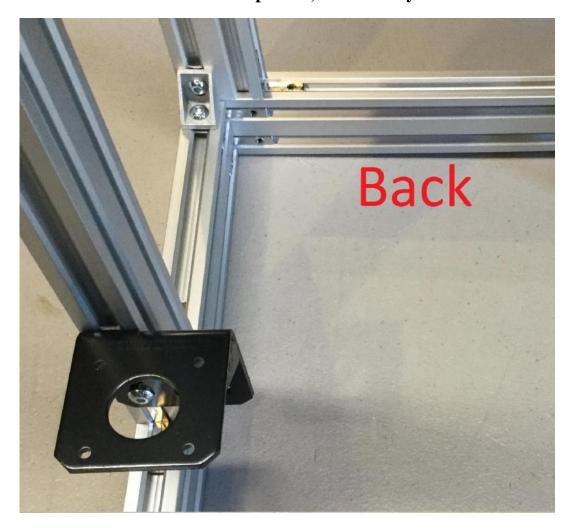
Next using the Extrusion, M5 bolts and T-Slot nuts install the extrusion into the cast corner brackets. Also install the M5x12mm bolt and T-Slot nut onto the right extrusion (Shown by red arrow).
