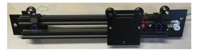
Install Two T-Slot Nuts into the Extrusion by the X Idler Bracket as shown by the Red Arrows Below, then install the Adjustable Z endstop piece with a M5x12mm bolt and T-Slot nut by the X motor bracket as shown by the Blue Arrow.
