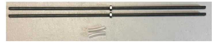
Thread the M5 nuts onto the threaded rods about half way, if the nut won't easily thread onto the threaded rod try the other end of the threaded rod.
