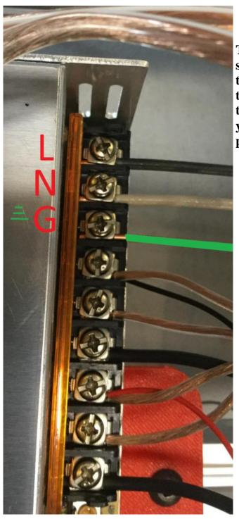
To connect your Power Cord to the power supply you will connect the Ground Wire to the Terminal Labeled G on your Power supply, then the Neutral wire to the one labeled N and the Live wire to the one labeled L. To turn your printer on and off you will plug in the power cord and unplug the cord.
