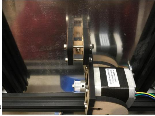
Now move the Heat Bed Mount to the front of the machine, align
