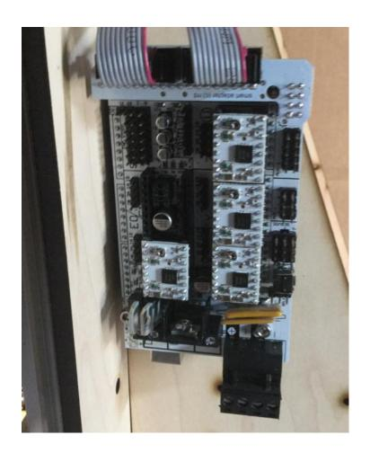
Next plug in the Endstops, make sure they are plugged in as shown or the printer will not power on.
