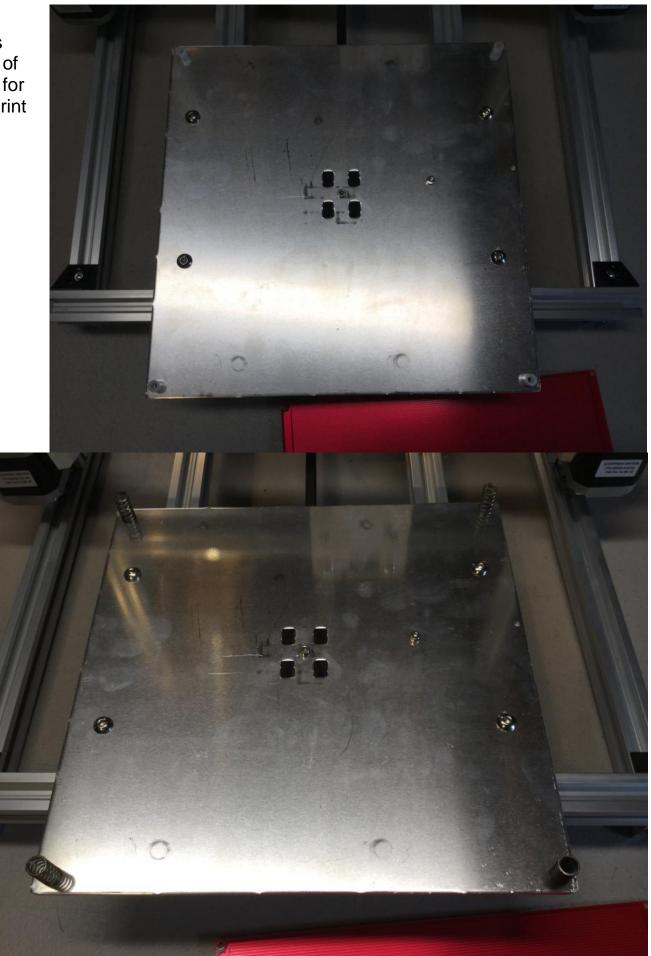
Install your Insulation/Fire Blanket on the heat bed mount, then put the heat bed on top then install 4 bolts through the corners, last install an M3 Nylon Lock nut onto each bolt and tighten them down.
