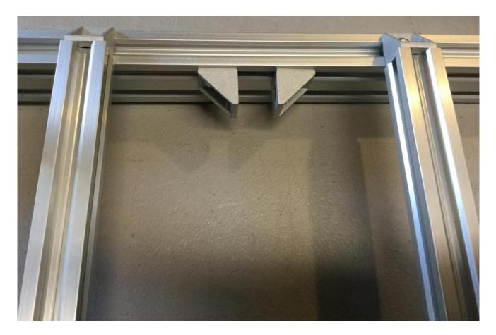
Make sure the bottom of the Extrusion is aligned with the bottom of the cast corner bracket on all 4 brackets otherwise your Y axis will not be flat.
