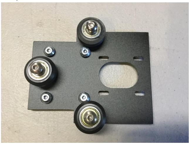
Flip the Metal plate back over, install a M5 washer on the bolt that has the eccentric spacer then install a Nylon M5 Lock Nut on the 3 Bolts and tighten
