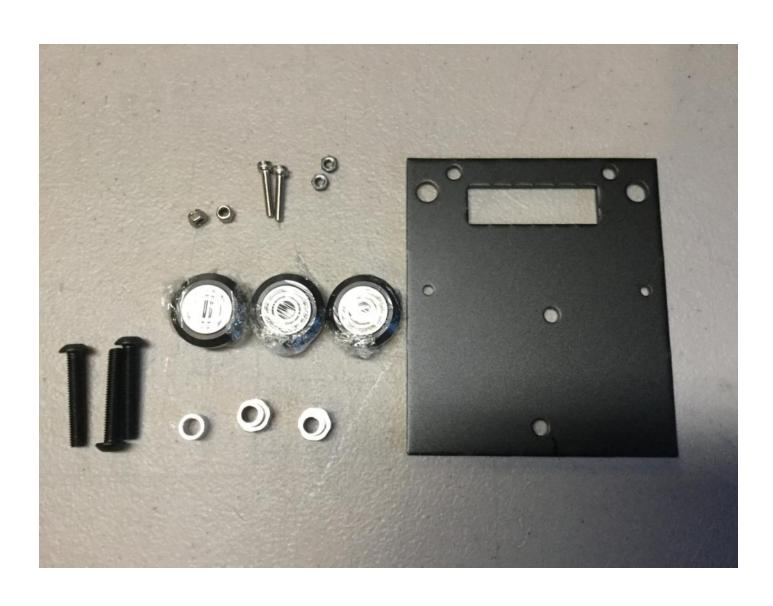
Position the X Carriage piece as shown in the picture on the right, make sure the hole shown with the red arrow is on the left. Install the 3 M5x30mm bolts as shown then install the Aluminum Spacer on the bottom bolt and the two eccentric spacers on the top two bolts. Push the eccentric spacer into the metal and turn them so the notch is on the top.
