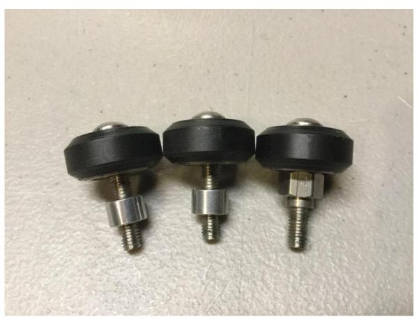
Flip the Metal plate over and install the two bolts with delrin idlers and aluminum spacers on the side closest to where the Motor mounts, then the one with the eccentric spacer on the left.
