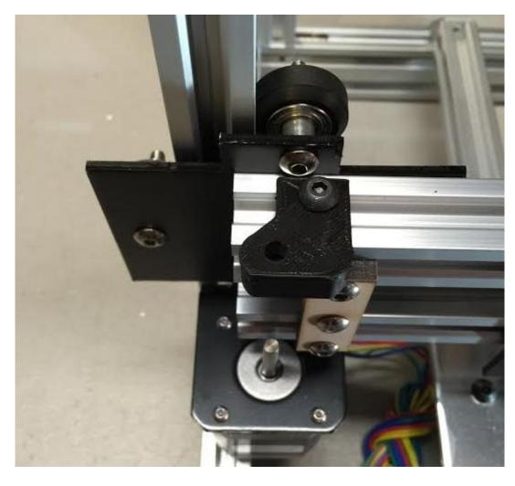
Next turn the printer upside down carefully and align the gears teeth with the wooden mount as shown in the picture, then tighten the gear down with a set screw
