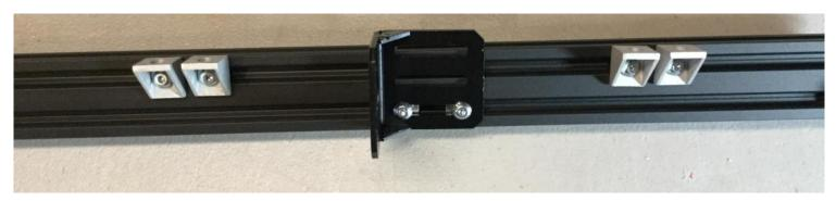
Now Install a Motor Mount of the right side of the printer, make sure you use the slot on the far left of the motor bracket.
