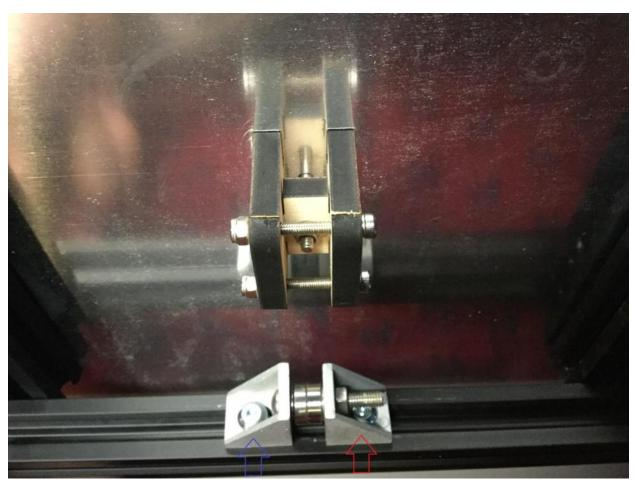
Now install the top of the frame onto the extrusions you just installed. For now you will just align the 8 hidden corner brackets on the top part of the frame with the 6 extrusions so make sure the hidden brackets move freely and are not bolted in place. Once you have the top frame on you can align the extrusion in the 4 corners and tighten down the hidden corner brackets (you may want to use a clamp if you have one to keep everything tight).
