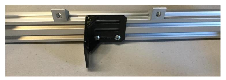
Now Install a Motor Mount of the right side of the printer, make sure you use the slot on the far left of the motor bracket.
