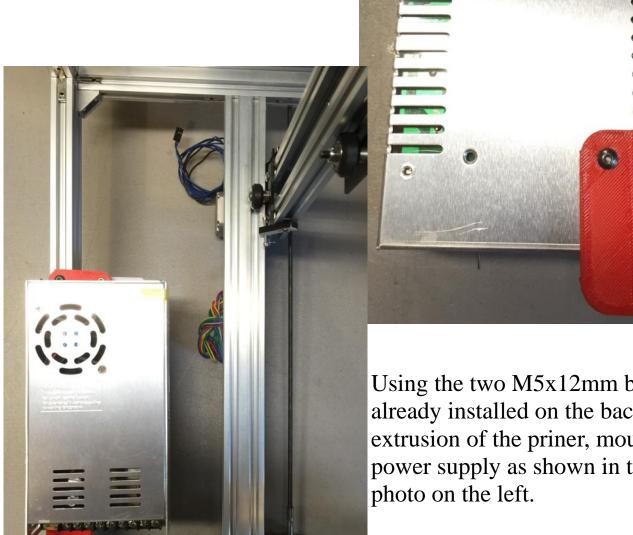
Using the two M5x12mm bolts already installed on the back right extrusion of the priner, mount the power supply as shown in the
