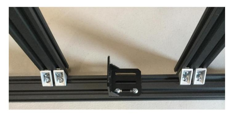
Make sure the bottom of the Extrusion is aligned with the top of the front and back extrusion pieces otherwise your Y axis will not be flat.
