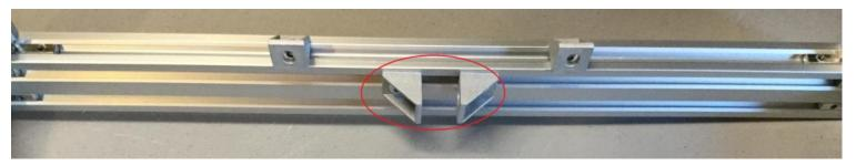
Now install 2 Cast Corner Brackets without Nubs and one Motor Mount on the bottom back of the frame using the previously installed M5x8mm Bolts. You will adjust the actually placement later.
