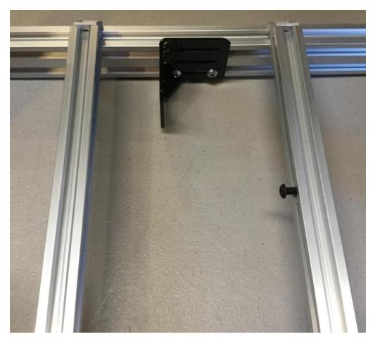
Connect the extrusion to the Cast Corner Brackets in the front of the machine also.
