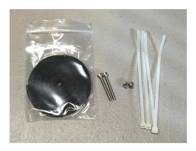
Next get your belt and cut a piece off that is 39 inches long loop one end over and use a zip tie to secure it, then install the belt through the Idler bearings.
