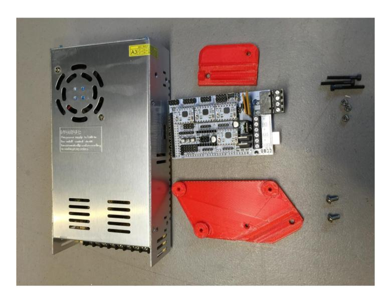
Install M3 nuts into the back of the printed mount as shown by the picture on the right, make sure the nuts are recessed into the mount.
