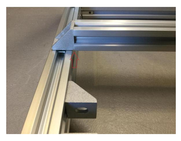
Install 6 Cast Corner Brackets on the bottom front of the machine using the M5x8mm bolts installed previously. You will adjust the actually placement later.
