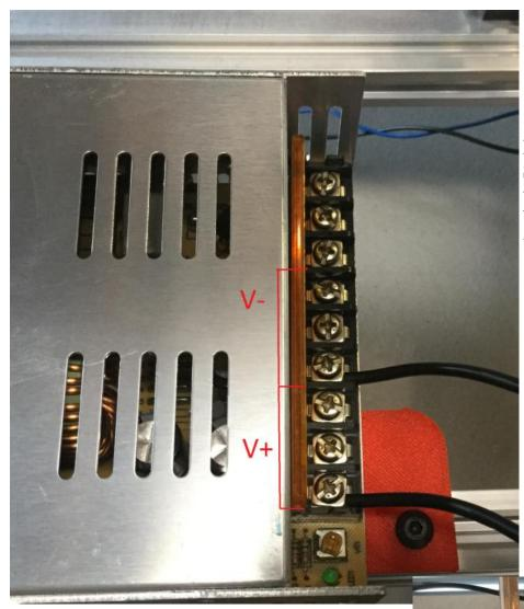
Connect your thick Heat Bed Wires to your Power Supply, Connect one wire to V+ and the other wire to V-, it doesn't matter which wire goes in either location.
