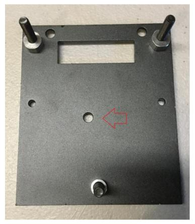
Install Delrin Idlers on to the 3 bolts then a M5 Nylon Lock nut onto each bolt, tighten the nuts, but make sure the Delrin Idlers still turn freely.
