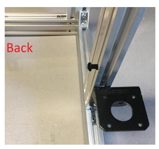
Now Install a Motor Mount of the left side of the printer, make sure you use the slot on
