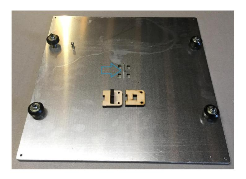
Now install the other A wood piece onto the + wood piece then install it into the Aluminum Heat Bed Mount and tighten it down with the M3 bolt and a Nylon Lock nut.
