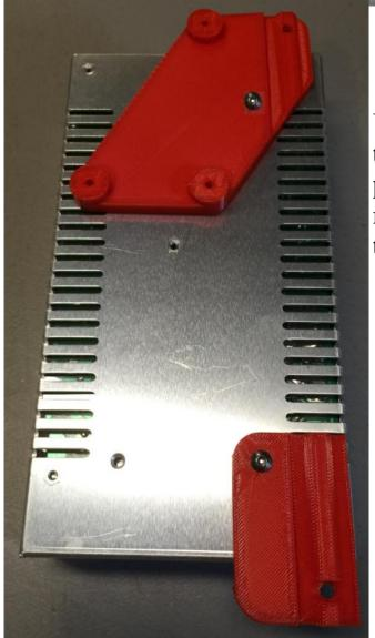
Using the two M4x8mm bolts mount the printed plates to the back of the power supply, the smaller plate will mount near the power connections for the power supply. Install the RAMPS onto the top printed mount using the 3 M3x25mm bolts, do not over tighten the bolts as that could damage the electronics.
