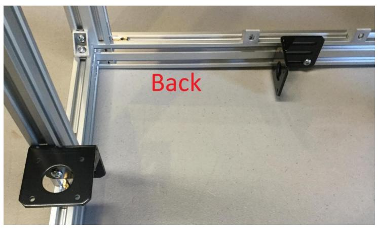
Next using the Extrusion and M5 bolts install the extrusion into the cast corner brackets. Also install the M5x12mm bolt and T-Slot nut onto the right extrusion.
